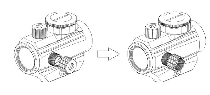
NOTE:Red dot sights need to be adjusted by instrument or aiming at a target of 30 to 50 yards (about 27 to 46 meters.) This is because the reflected rays are parallel to the rays seen by the observer, so using an instrument or actually aiming at the target can help to see the movement of the red dot more clearly.
